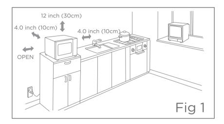
A 10-cm spacing should be kept between the appliance and right and back walls, and a 30-cm spacing kept on the top. Never dismantle the applicance's feet, nor block the air intake and exhaust opening. The left side must be open.
